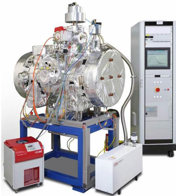
Fig. 36: Photo of the test tank for injection kicker with heating jackets, pumps, and control rack.
